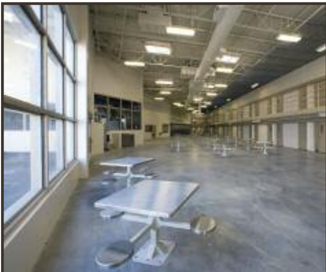
This is an interior shot of the dayroom in one of the four identical close-custody housing units. To the left is a large security glass panel to bring natural light into the dayroom.
